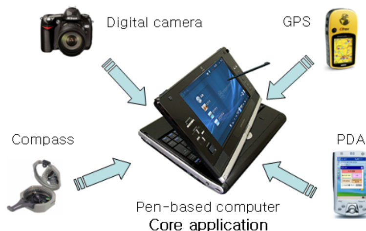
Figure 1. Components of a real-time pen-based data collection system (Nguyen, 2008)
